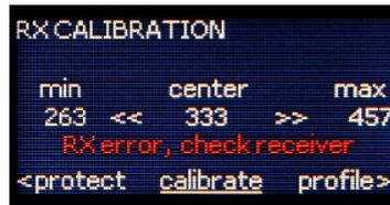
For radio system calibration, choose the RX CALIBRATION in the **Blue menu** (Setting 1) using the buttons. Press calibrate button and hold it for approx. 1s. Push full throttle, full brake and return to neutral. Then press the Ok button. The calibration is done.
