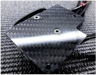
An example of NITRIDE installation into 4WD using the graphite plate screwed into the chassis of the car
