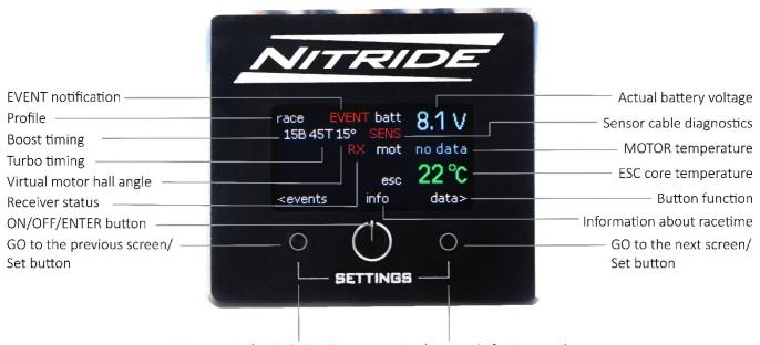
To enter to the Main Settings press simultaneously for 2 seconds.
