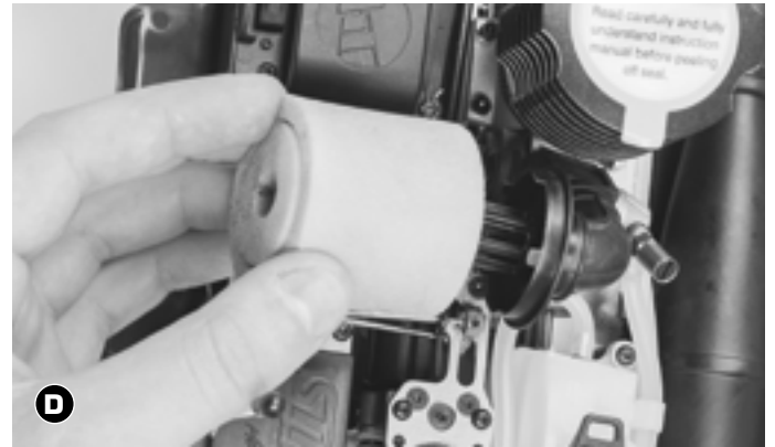
D Install the double air filter foam on it's holder with the provided wrench
