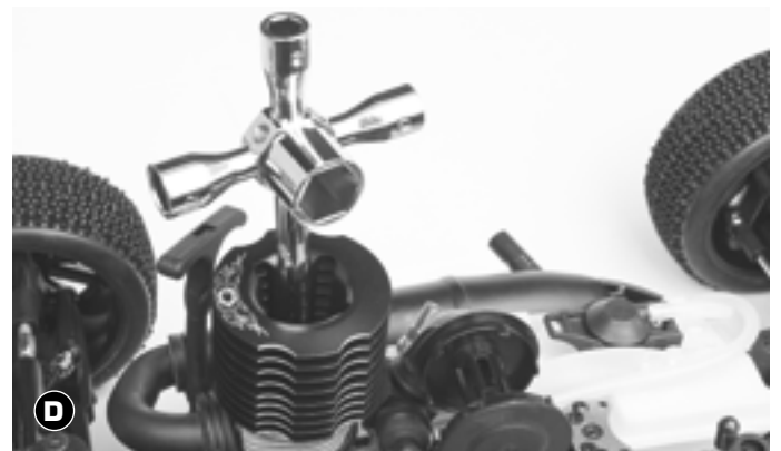
D Screw up the glow plugs until the maximum and tighten weel
