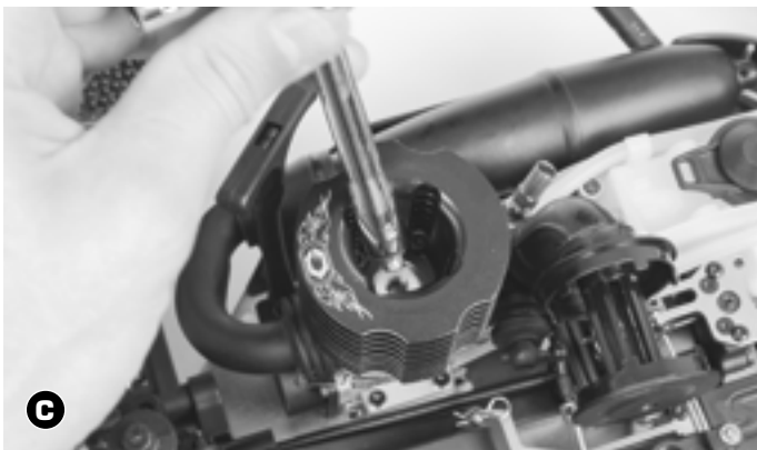
C Use the wrench to screw the glow plugs carefully into the engine burn room
