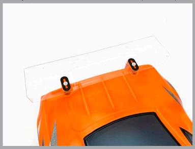
Place another Prescision Carbon Wing Mount Plate inside of the Bodyshell. This extend the rigidy of the mount and keep the screw in the correct position, which is even more important if you drilled additional holes.
