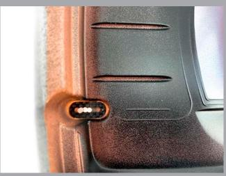
Depending on the Bodyshell thickness (\*2) its possible to drill the holes right after each other. We highly recommend to use the Precision Carbon Wing Mount plates on the in and the outside! The form fit of these plates inside the wing mount will ensure a perfect and stong bolting of the wing.
