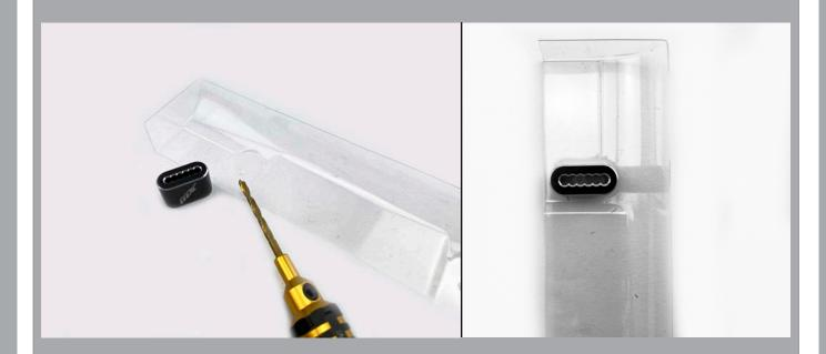
Remind the orientation of the drill jig! Take care to insert the drill bit correctly otherwise it could bind or you even damge the aluminum jig.
