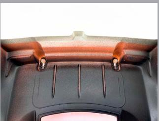
Keep the position of the screw in the outer top plate of the wing. It only needs to be changed in case you drill another hole in the wing itself.
